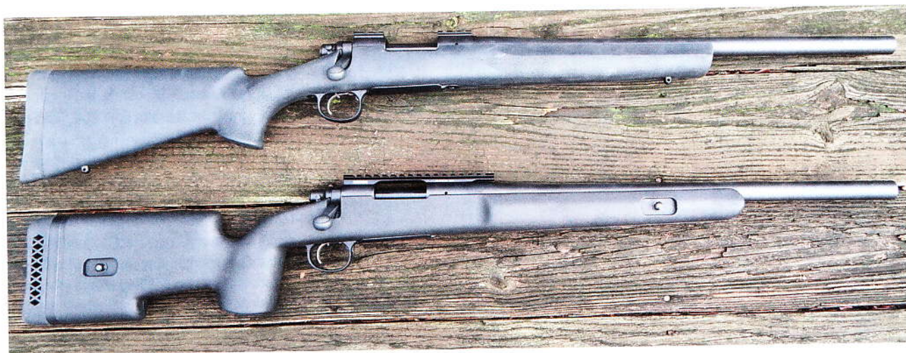
An upgraded tactical stock—to one that won't ever touch the barrel, is a great place to start your customization.
